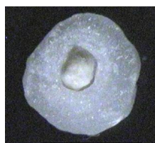
Urea particle containing 3% zinc core granule cross section
